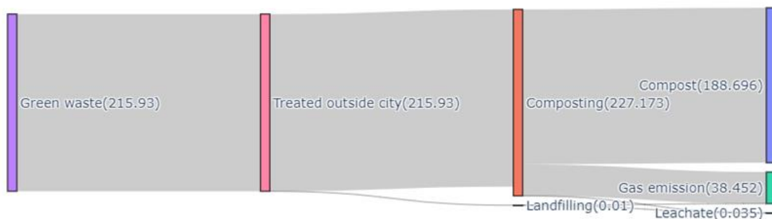
Figure E1. Sankey diagram of waste flows of green waste from Leicester City, the unit is tonnes.
