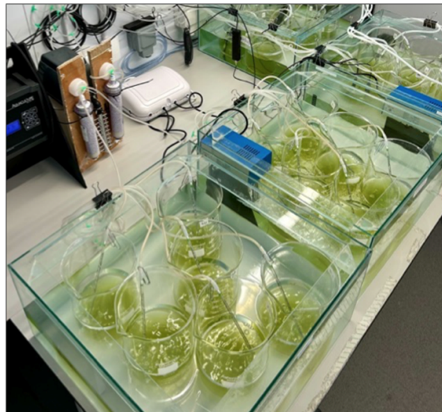
Figure 11: Experimental setup with phytoplankton culture containers (microcosms) used to test the effects of \text{CO}_2 leakage and warming on phytoplankton communities.
